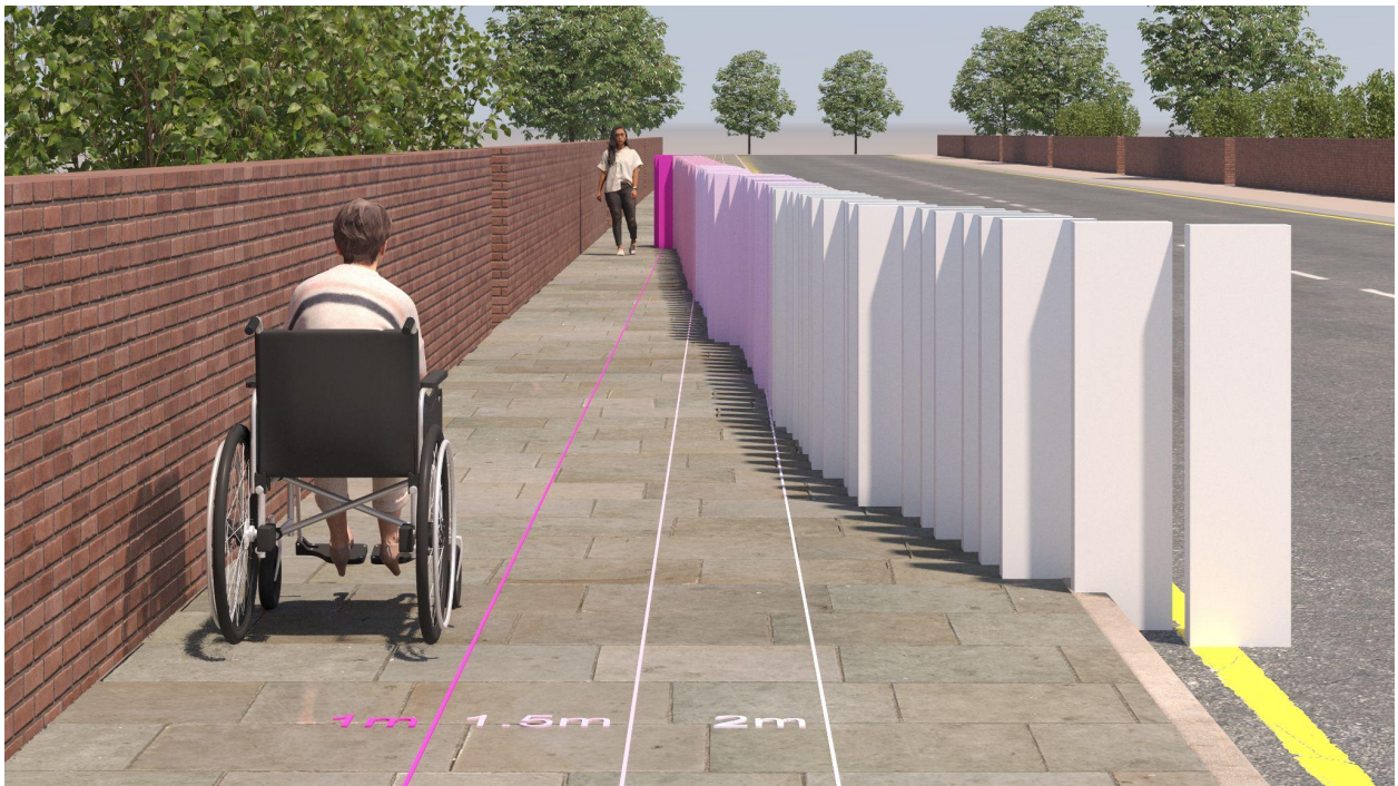
Figure 17: clear footway width at pavement installations of EV chargepoints in the London Borough of Hammersmith & Fulham, January 2023
